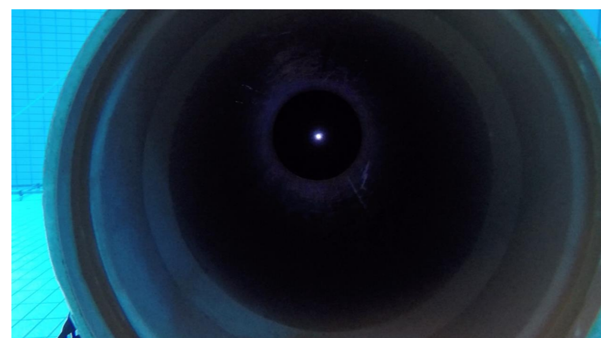
Figure 1: Light-shielded tube was used for CFFF in dark conditions both on land and underwater. Participants' view into the tube. Light source at the end (1.5 m)
