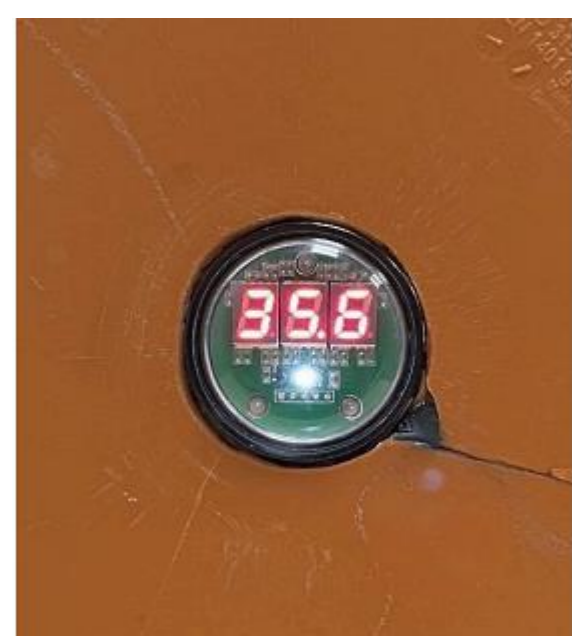
Figure 2: Flicker Tool as seen by the participant. The Flicker value is not visible during testing
